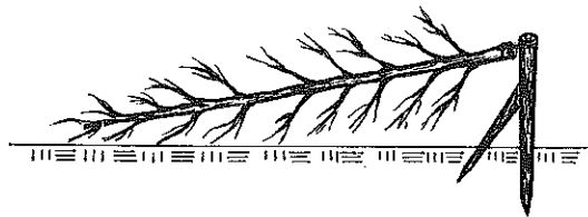
Fig. 55: Anchoring of tree in the Rauhbaum method
