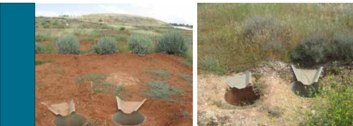
Figure 48. Measurement of runoff from exposed and treated areas at the ICARDA compound in Aleppo, Syria
