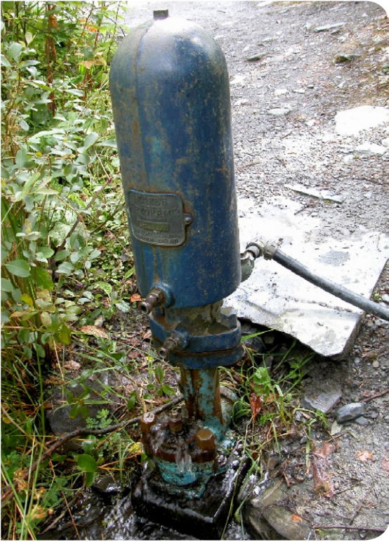
Figure 6 Hydraulic ram pump (Wikipedia.org)
