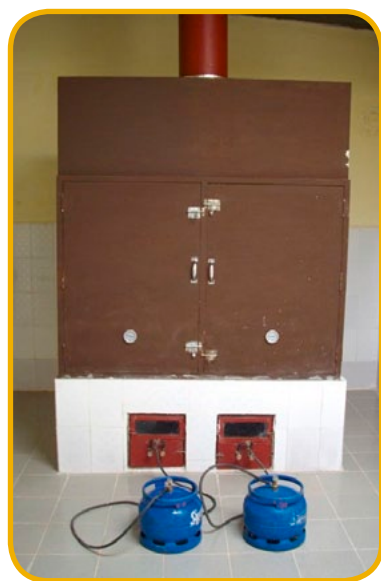
Photo 66: Operational gas dryer
