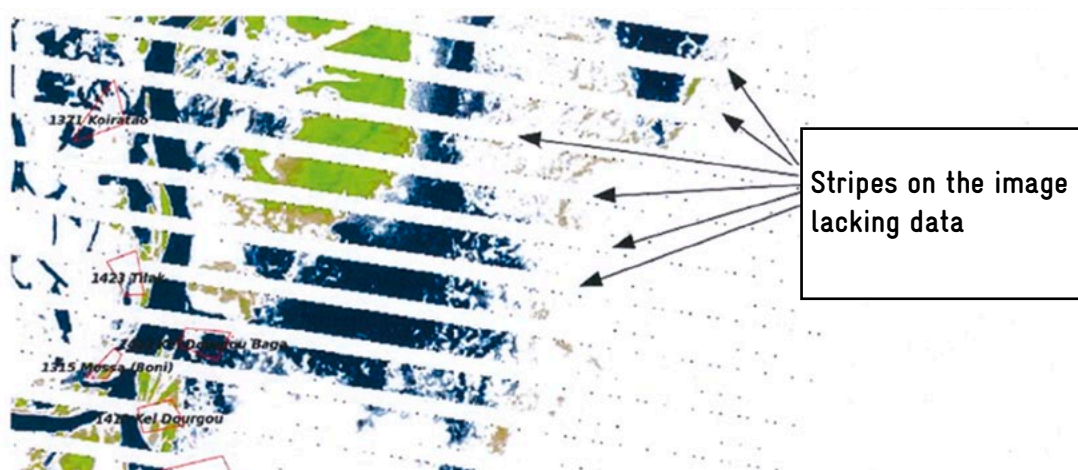
Figure 3: Landsat 7 image with stripes
