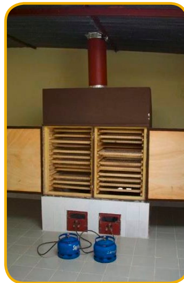
Photo 67: Unfilled gas dryer
