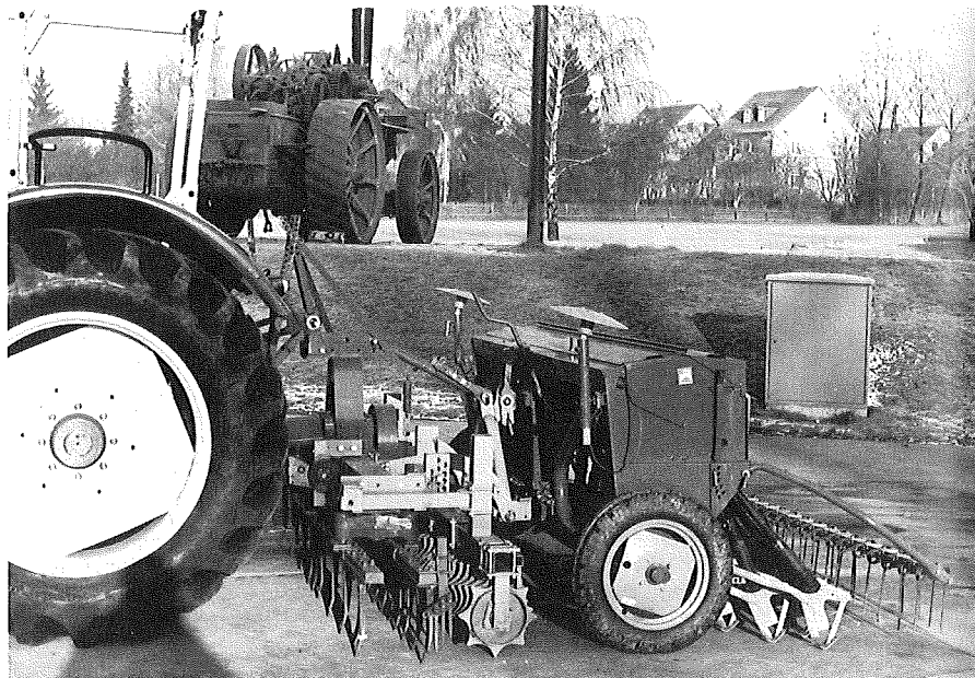
Fig. 87. Reciprocating hoe with rear-mounted drill.
