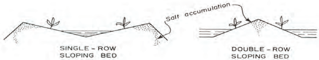
Fig.21. Salinity control with sloping beds irrigating on both sides of the furrow (source: Water quality for agriculture)
