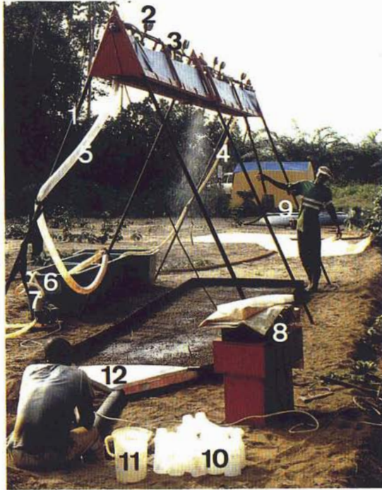
Figure 612-1: Mobile rainfall simulator unit in the field. 1: simulator; 2: manometer; 3: spraying nozzle; 4: supply hose; 5: outlet hose; 6: 300 l tanks; 7: electric pump; 8: electronic control system; 9: 5000 l tank; 10: 1 l sampling bottles; 11: 5 l beaker; 12: outlet; 13: disassembled simulator; 14: 120 l barrels for water transport
