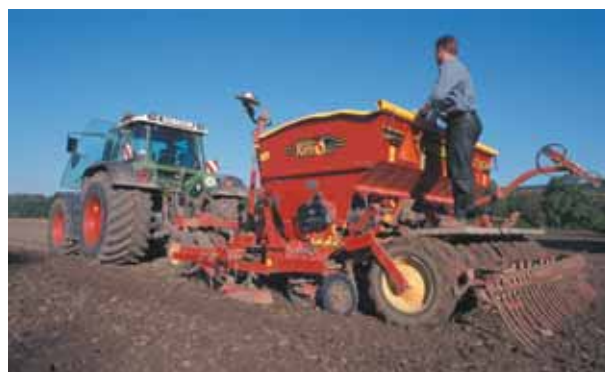
A direct seeding machine in operation. Residual seed can be completely removed from seeding machines relatively easily.
