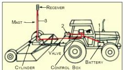
The laser levelling process starts with a field survey for determining the level or slope of the plot as well as surveying the high and low spots in the field. For successful automated operation, the difference between the high and low spots should not be greater than 15 cm for one pass. Otherwise the transmitter must be set twice and a second pass would be needed.
