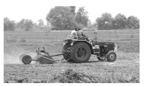
The availability of tractors equipped with a hydraulic command system in the 1980's made it possible to use hydraulically operated implements. Unlike the grading buckle described before, this type of leveler is attached to a tractor by means of a long dragbar. The leveler is equipped with a hydraulic piston to adjust the position of the shield or buckle. It is equally possible to tilt the shield or buckle. This option overcomes the incon-
