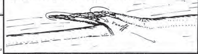
Fig 9 Ditchira Bund (adapted from SNNP region)
