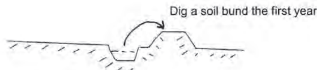
Fig 4 Upgrading of soil bunds using the fanya juu principle after 1-2 years from construction
