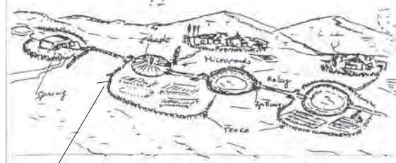
Relay microponds storing high overnight flow (linked by stone paved waterways)
