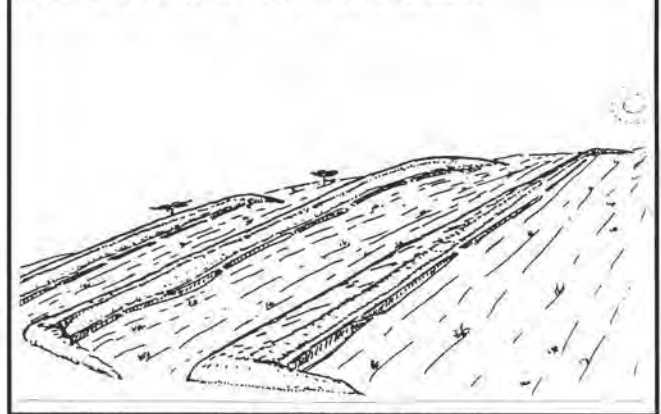
Fig 3 Reinforcement of bunds in slight depression points (lateral slopes within plot)
