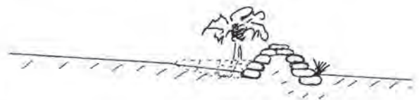
Fig 3. Double faced stone/soil bunds without collection trench suitable in sandy soils and uniform terrains (<8% slope)
