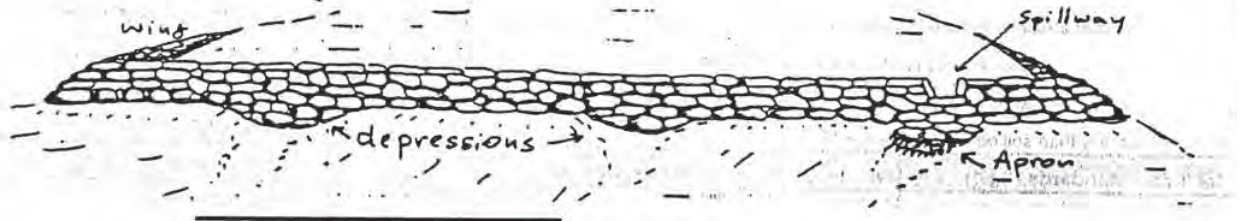
Fig 2. Bunds that cross depression points without following exact contour lines: Reinforcements at depression points + keys
